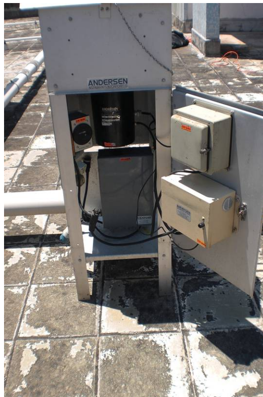
High-Volume Dust Sampler
